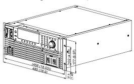
When mounting on a millimeter rack (bracket model KRB200)
