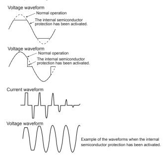
In AC mode, you can set the time that elapses after the internal semiconductor protection function is activated before an alarm is generated. An alarm will only be generated if the internal semiconductor protection function circuit remains activated continually for the specified length of time. This is useful when you don't want alarms to be generated due to short-term overloads such as those caused by inrush current.
