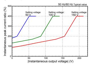
Fig.11 Instantaneous output voltage ratio versus instantaneous peak current ratio (AC mode H range, excluding threephase three-wire output)
