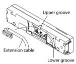
Slide the connector cover back onto the control panel.
