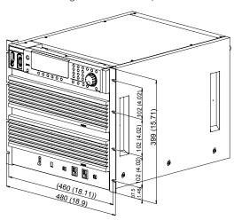
When mounting on a millimeter rack (bracket model KRB400-PCR-LE)  $\,$
