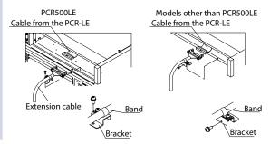
Connect the control panel extension cable to the control panel.
