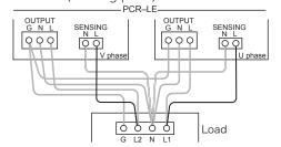
Three-phase output (Three-phase four-wire)
