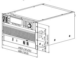
When mounting on a millimeter rack (bracket model KRB300)
