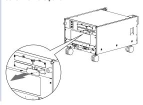
Hold the panel parts of the board so that the printed circuit board side is facing up.
