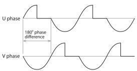
If you want to use two-phase such as in a V wiring connection, set 2P Mode to ON.
