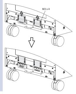
Remove the two terminal block tray screws, and then pull the tray out.
