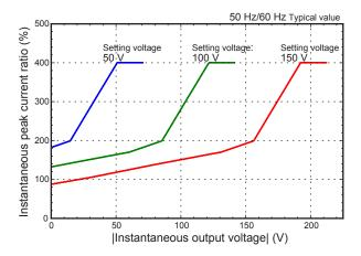
■ Fig.6 Instantaneous output voltage versus instantenous peak current ratio (AC mode H range, excluding three-phase three-wire output)
