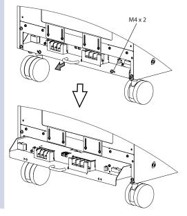
Pull out the stopper to lock the terminal block tray in place.
