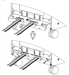
Slide the two terminal box covers down until they are touching the wires, and then use the four screws to fix the terminal box covers in place.
