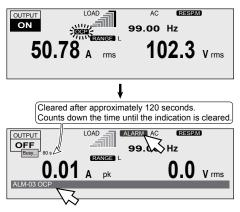
If the internal semiconductor protection is activated repeatedly, the PCR-LE Series may malfunction.
