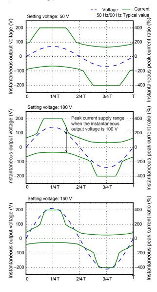
Fig.13 Voltage waveform versus peak current supply range (AC mode H range)
