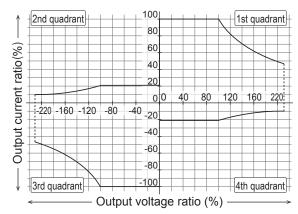
If you use the PCR-LE Series with a current that exceeds the rated DC output current, the protection functions will be activated, which may cause the output voltage to drop or turn off the output.
