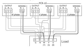
· Three-phase output (Three-phase three-wire)
