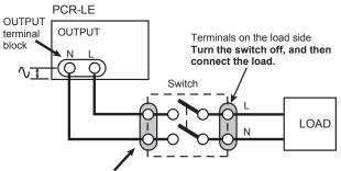
Terminals on the OUTPUT terminal block side Risk of electric shock. Do not touch the terminals.
