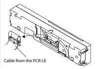
Connect the cable from the PCR-LE Series to the control panel extension cable. Use the band and the bracket to fix the control panel extension cable to the PCR-LE Series.
