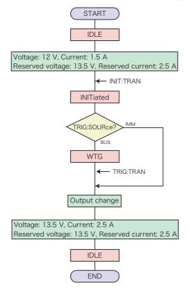
The TRIGger:TRANSient:SOURce command sets the trigger source to BUS, or IMMediate
