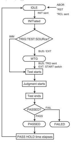
SEQuence2 (TEST) trigger function flowchart
