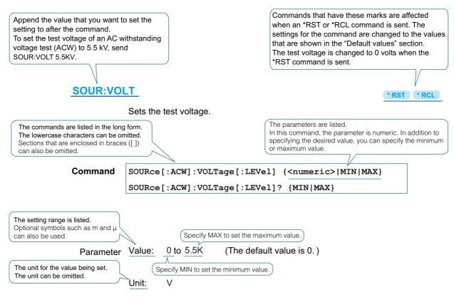
Response Returns the test voltage in <NR3> format.
